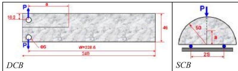
**Fig. 1: Geometry and loading conditions of SCB and DCB specimens subjected to mode I loading (dimensions: mm).**
